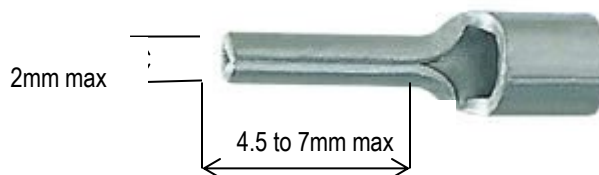
2-15. Lead Terminal for TEC-2400
