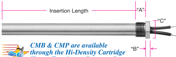
TYPE CM Fig. 1 – Fitting Flush with Lead End of Sheath
