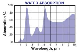
**SPECTRAL NATURE:** To address this issue, heaters should be designed to emit wavelengths that closely match the absorption band of the processed material in a given application. By carefully considering the broad side-bands of the emitted radiation and absorption, it is possible to design systems that will enhance the heat transfer rates at different stages of the heating process.
