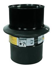
You should not be heating heat sensitive materials with Model TRX-55. Heat the material to the desired temperature then turn the control back (c.c.w.) to the point where the thermostat just turns off as indicated by the red pilot light no longer glowing. The control will maintain the desired temperature within plus or minus twenty degrees Fahrenheit.
