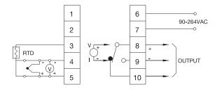
NOTE: Terminals 8, 9 and 10 are not used for Model TEC-900.
