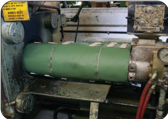
Tempco offers a line of Modular Insulating Blankets designed to contain the heat generated by industrial elements in various applications, thereby conserving energy and cooling the environment.
