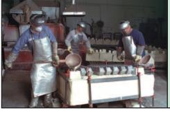
Processing aluminum castings using a Sand Mold.
