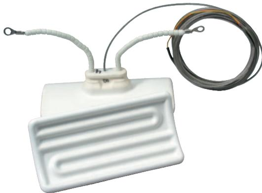
Designed for use in the CRB, CRC, CRL, CRG and CRM solid curved and flat face style heaters. Low noise thermocouples can only be factory installed and must be specified at time of ordering.
