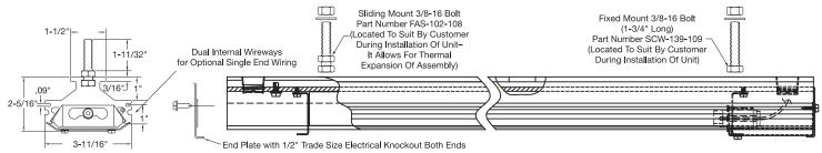
**Danger: Hazard of Fire** Do not mount heater closer than 6" to any combustible or structural material that does not have at least a 200°C continuous temperature rating.
