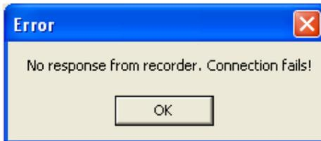
If this is the case, please check the Ethernet cable connections at both the recorder and PC/LAN HUB side. Also make sure that green communication LED available for proper firm connection at RJ 45 connector.
