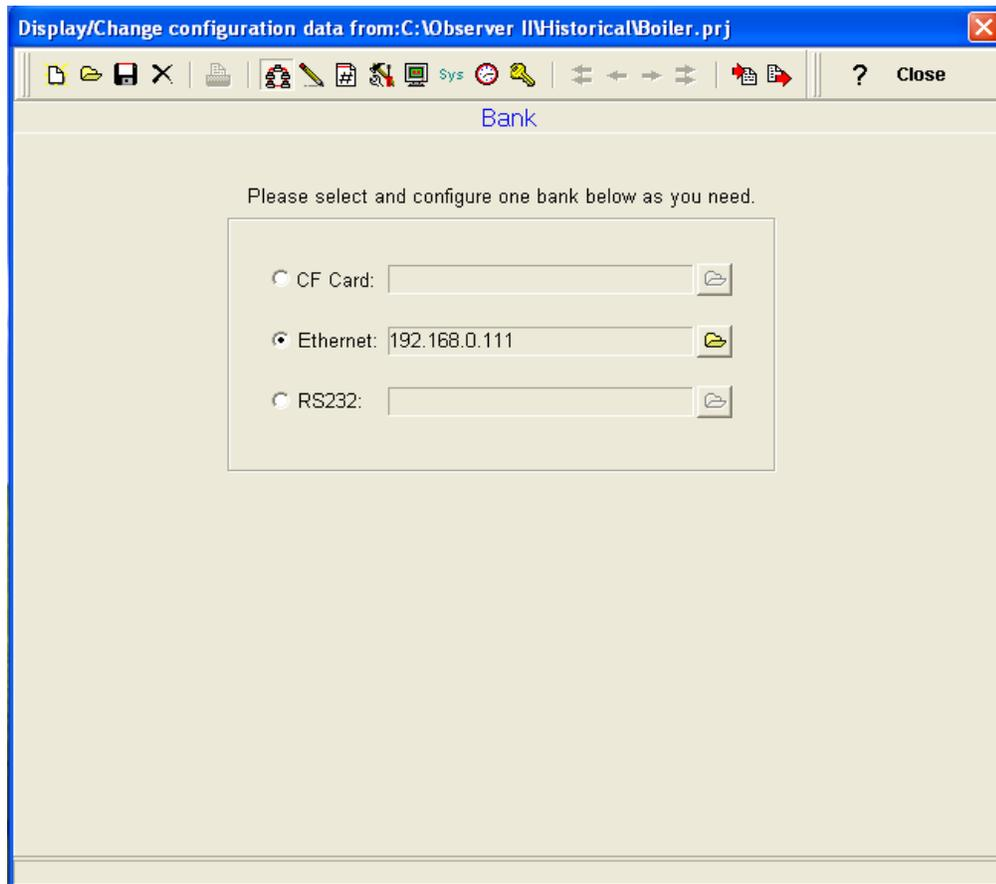
32 MB CF card shall be supplied along with the recorder. Standard Ethernet port (RJ 45 female) shall be available at the recorder. RS 232/ RS485 shall be supplied as additional options.
