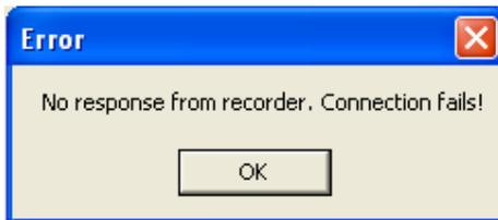
If this is the case, please check the RS 232 cable connections at both the recorder and PC. Also make sure that green communication LED available for proper firm connection at back RS 232 port available at recorder back side.
