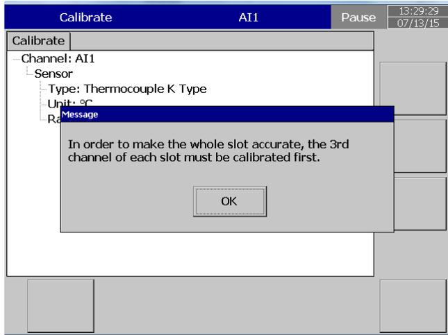
Click OK and proceed and select the channel of Analog Output to be calibrated.
