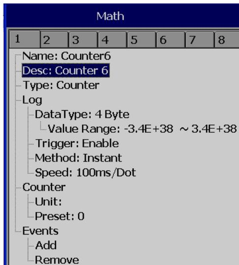
Press directional keys < > at the bottom to select one of the Math channels for the Counter operation.
