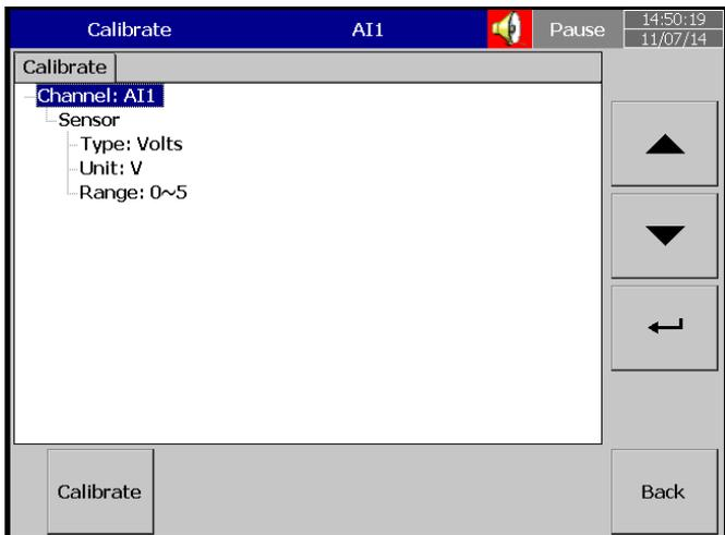
Please note that, in order to calibrate the whole Module slot accurately, the 3rd channel of each slot must be calibrated first. Click OK.
