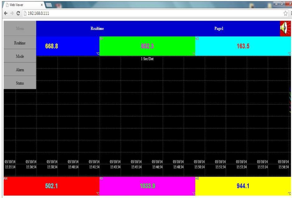
The display includes Real time values of all channels like AI, Math, Counters, Totalizers, Real time alarms, historical alarms, status of Digital Inputs, Digital Outputs, Analog Outputs, Counters, and Totalizers etc.
