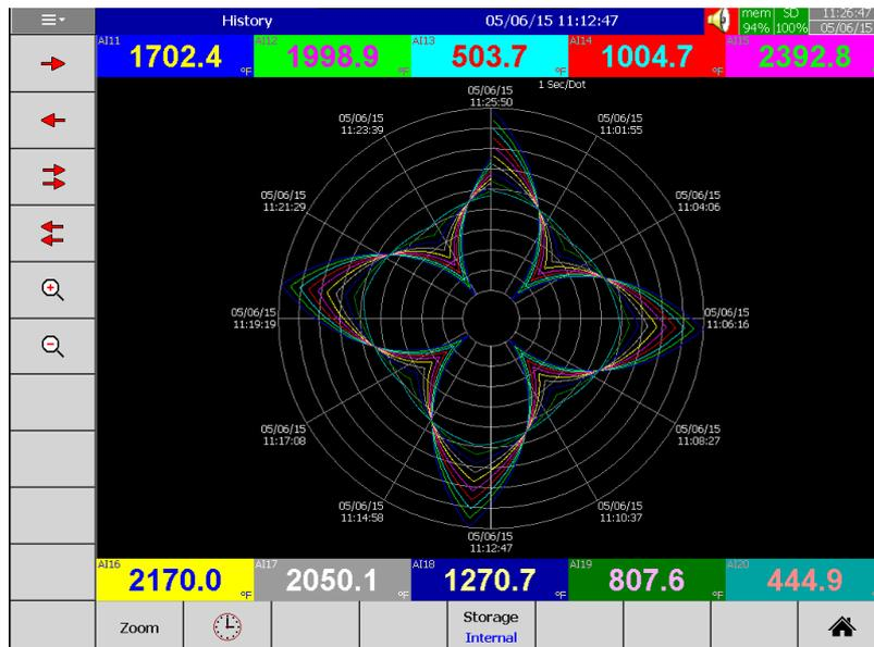
**Speed:** This is the display speed. Available options are 100 msec/dot, 1 Sec/dot, 2 Sec/dot, 5 Sec/dot, 10 Sec/dot, 20 Sec/dot, 30 Sec/dot, 1 min/dot, 5 min/dot, 10 min/Page, 30 min/Page, 1 hour/Page, 2 hour/Page, 4 hour/Page, 8 hour/Page, 12 hour/Page and 1 Day/Page.
