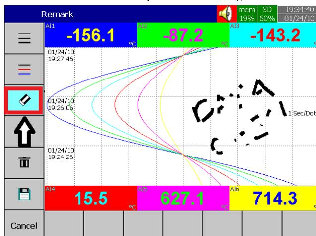
If the User wants to undo part of a message, he/she can do this by pressing the undo symbol (shown in the red box in the picture below). This will undo the last part of the message.
