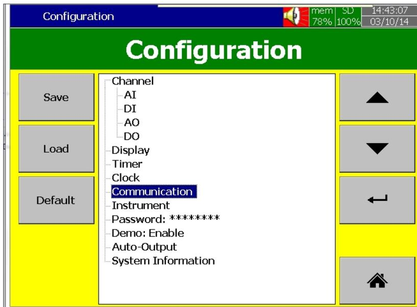
After completing the above steps, press the "BACK" key, then the "Home" key to return to the main menu. It will save the configuration settings in the Recorder.
