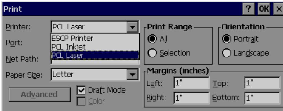
**Printer:** PCL Laser, ESCP printer, PCL Inkjet available by default. Select one from the list as per printer model connected to the Paperless Recorder
