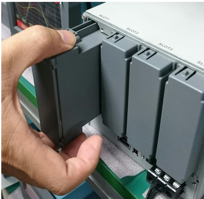
**Note 4:** For the PPS-3000, Analog Input card should be inserted in slots 1 to 8 only.
