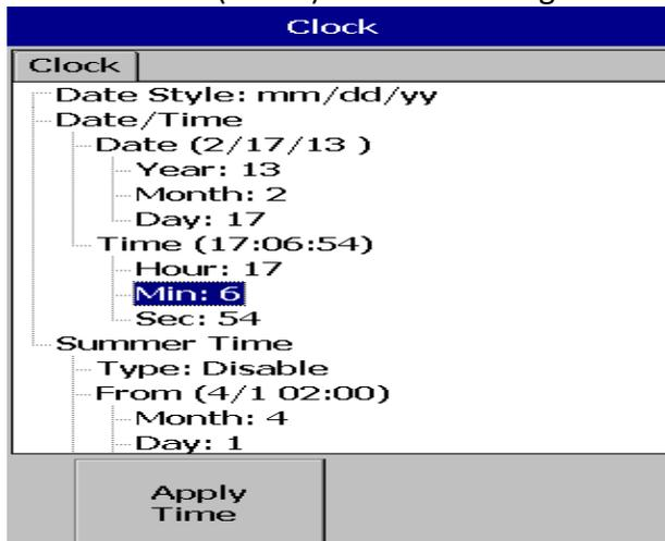
Fig: Clock configuration page in Paperless Recorder
