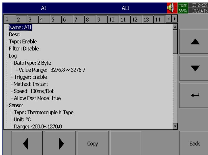
**Copy:** For example, to copy the channel configuration from channel 1 to channel 2, select the source channel, in this case AI1 (or whatever the channel is named), press on “Copy” button. Now, a “Paste” button will get enabled, go to target channel, say channel 2, and then press on “Paste” button.
