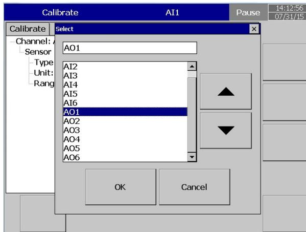
Confirm the channel to calibrate and click "Calibrate" and "yes" in the next screen
