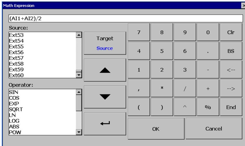
The Source covers all available Analog inputs, Digital Inputs, Math inputs, external channels.
