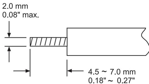
Figure 2.2 Lead Termination
