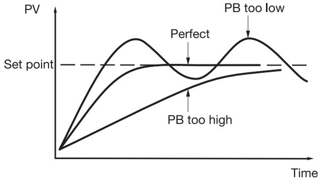
**Figure 3.25 Effects of PID Adjustment**
