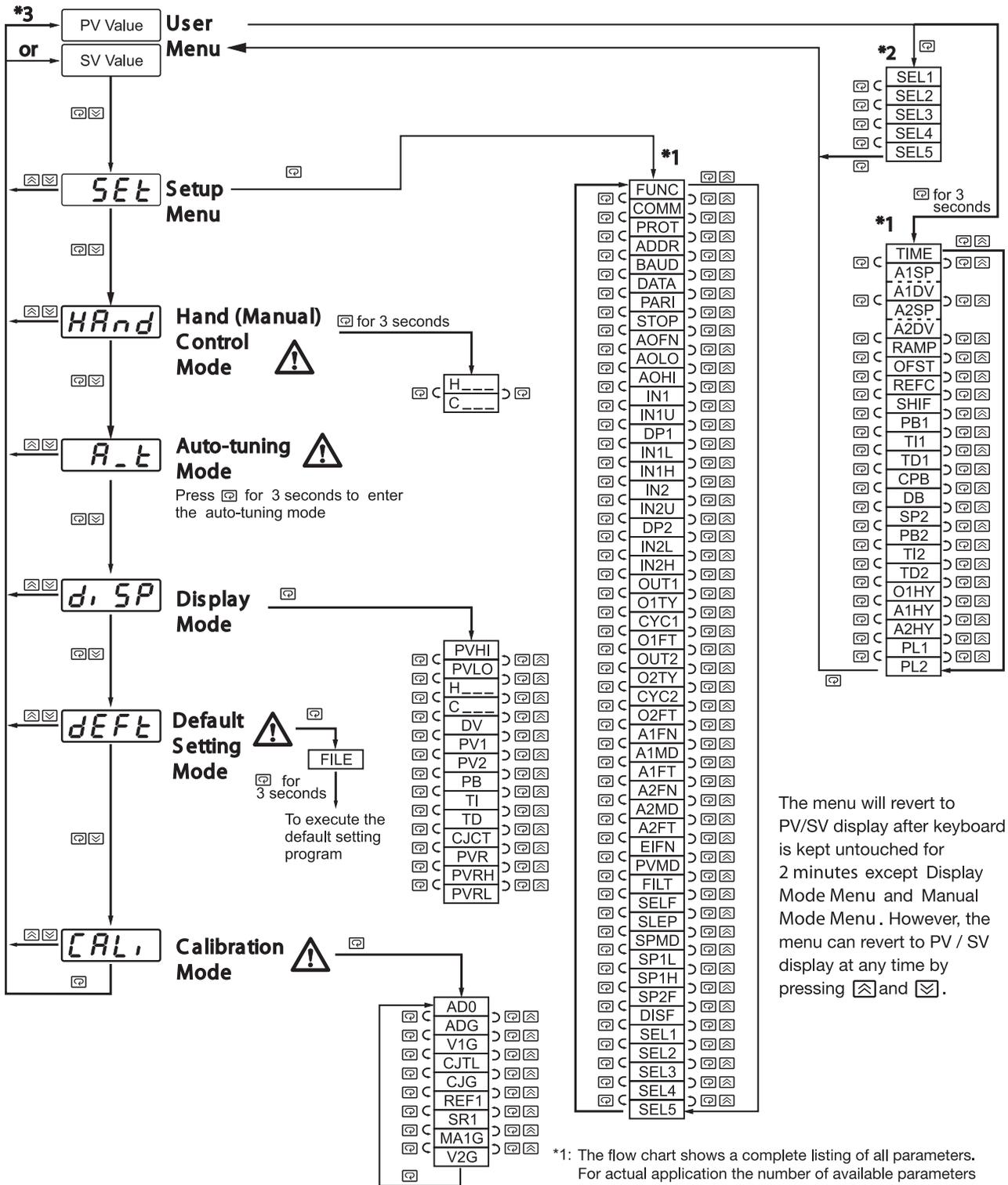
The menu will revert to PV/SV display after keyboard is kept untouched for 2 minutes except Display Mode Menu and Manual Mode Menu. However, the menu can revert to PV / SV display at any time by pressing **☐** and **☐**.
