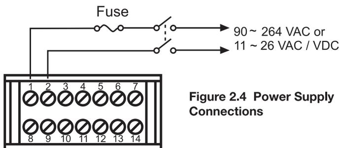
Figure 2.4 Power Supply Connections
