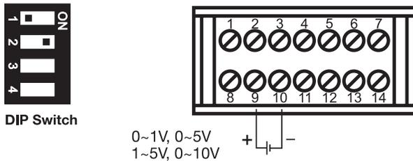
Figure 2.7 Input 1 Linear Voltage Wiring
