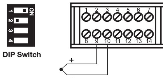
Figure 2.5 Thermocouple Input Wiring
