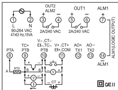
Figure 2.3 Rear Terminal Connection Diagram
