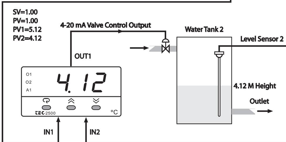
Adjust SP (here it is 1.00) to control the difference between PV1 and PV2. Choose P1-2 for PVMD; the PV display will show the difference value (PV1-PV2) between PV1 and PV2, and this value will be stabilized at the set point (here it is 1.00). If you need PV1 or PV2 instead of PV, you can use the display mode to select PV1 or PV2 for display. See section 3-24. The above diagram indicates PV2 instead of PV.
