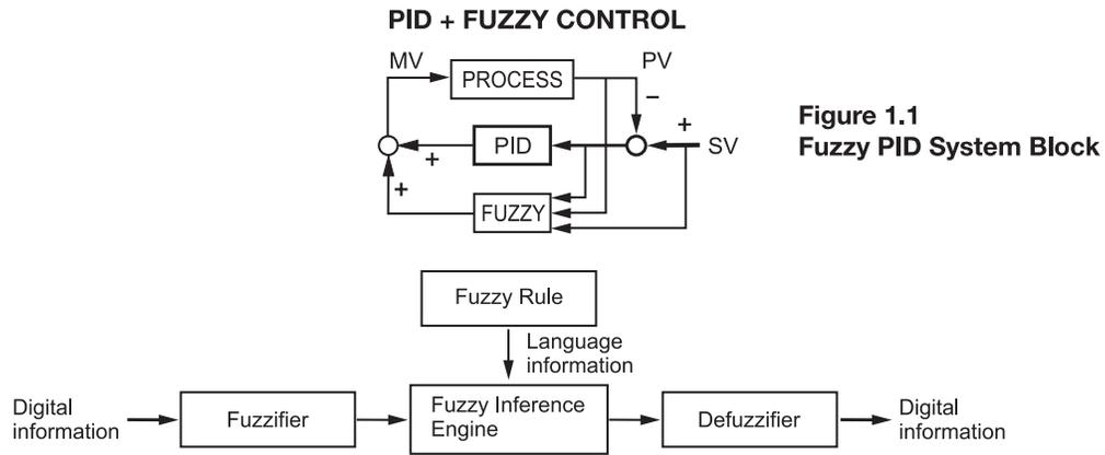
The function of Fuzzy Logic is to adjust PID parameters internally in order to make manipulation of output value MV more flexible and adaptive to various processes.
