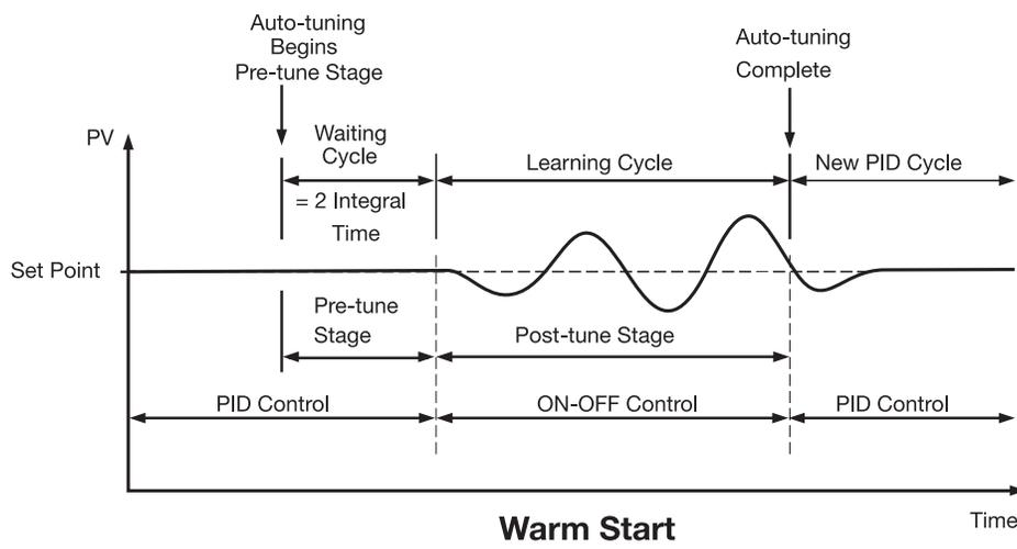
If auto-tuning begins near the set point (warm start), the unit skips the warm-up cycle and enters the waiting cycle. Afterward, the procedures are the same as described for cold start.
