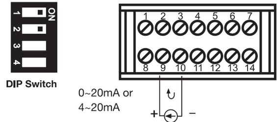
Figure 2.8 Input 1 Linear Current Wiring
