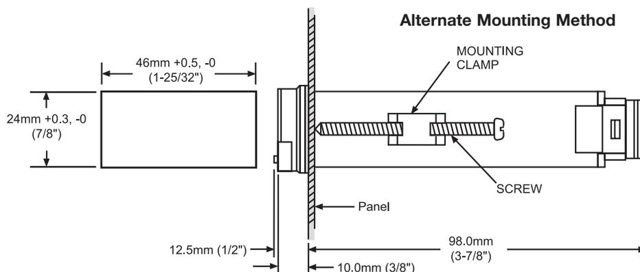
Figure 2.1 Mounting Dimensions
