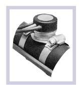
This control is a preset, epoxy-sealed thermostat containing a hermetically sealed single pole, double throw switch with normally open and normally closed connections
