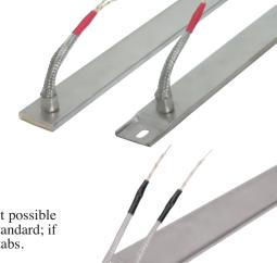
Type W2 Stainless steel braid over each lead wire offers sharp bending not possible with armor cable, as well as abrasion protection. 10" long leads standard; if longer leads are required, specify. Not available on heaters with tabs.
