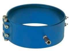
A standard Bayonet Adapter facilitates the installation of an external thermocouple with a standard bayonet cap. The standard location for the adapter is 90° from the gap.
