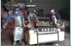
Processing aluminum castings using a Sand Mold.
