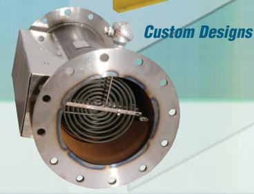
Duct Heater System: Tempco can supply the heater and blower assembled, ready for connection to the application duct work. The pictured 48KW, 480V unit produces 1500 CFM of heated air to dry metal parts after being coated with a rust inhibitor.
