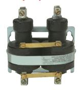
**Tempco's Mercury Displacement Relays** are specifically designed for resistive loads typical of heating and process equipment. These mercury relays are available in 35 and 60 amp models with single, double and triple pole configurations. Coil voltages range from 24 to 480 Volts AC at 50/60 Hz and 24 Volts DC.
