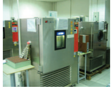
Environmental Test Chamber for Product Burn-In
