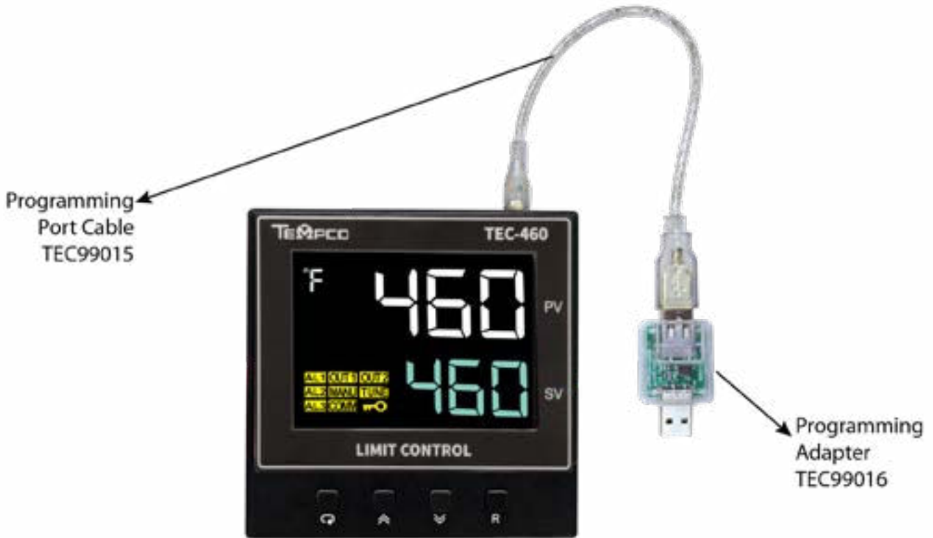
Figure 1-2 Programming Port Connection with Programming Port Adaptor
