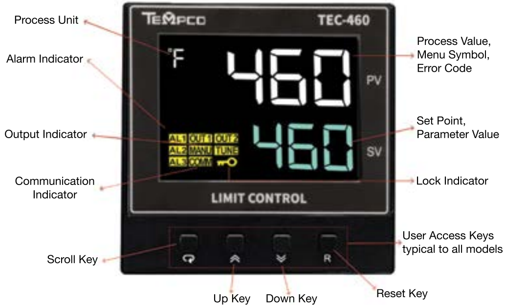
Figure 1-3 TEC-460 Front Panel Keys and Display 1/4 DIN
